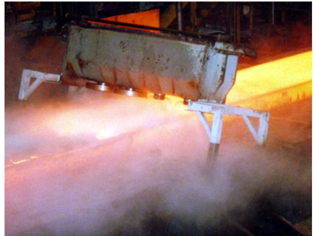
Figure 3: Rotor Descaler Trials at the Hot Strip Mill of VOEST-ALPINE STAHL LINZ
